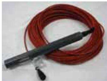
*Digital Hydrocarbon Probe (DHP-485)*
