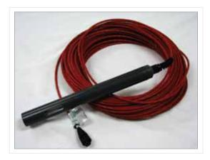
PetroSense **DHP probes** combine FCI's patented fiber optic chemical sensor (FOCS®) technology with digital electronics and an advanced microprocessor to make these products unique in the marketplace. FOCS technology is based on modulation of the transmitted light intensity when the sensor is exposed to hydrocarbons.
